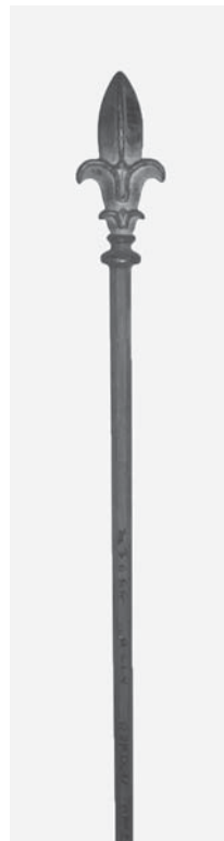
R155 H1410mm Bar: Octagonal W25mm Finial: H200 x W100mm Cl:6.7kg Alu:2.4kg
