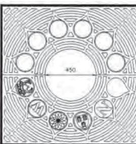
G150A 1220 x 1220 x 350 x 20mm Thick Cl:102kg
