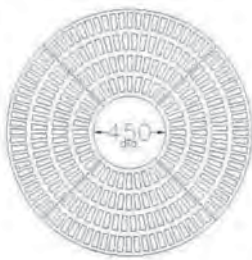
G004 1525 O/D x 450 x 600 I/D x 25mm Thick Cl:127kg
