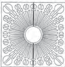
G012A 1000 x 1000 x 350 I/D x 25mm Thick Cl:94kg
