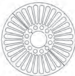
G005A 2000 x 450 I/D x 20mm Thick Cl:94kg
