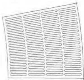
G000 11120 O/D x 8920 I/D x 25mm Thick Cl:99kg
