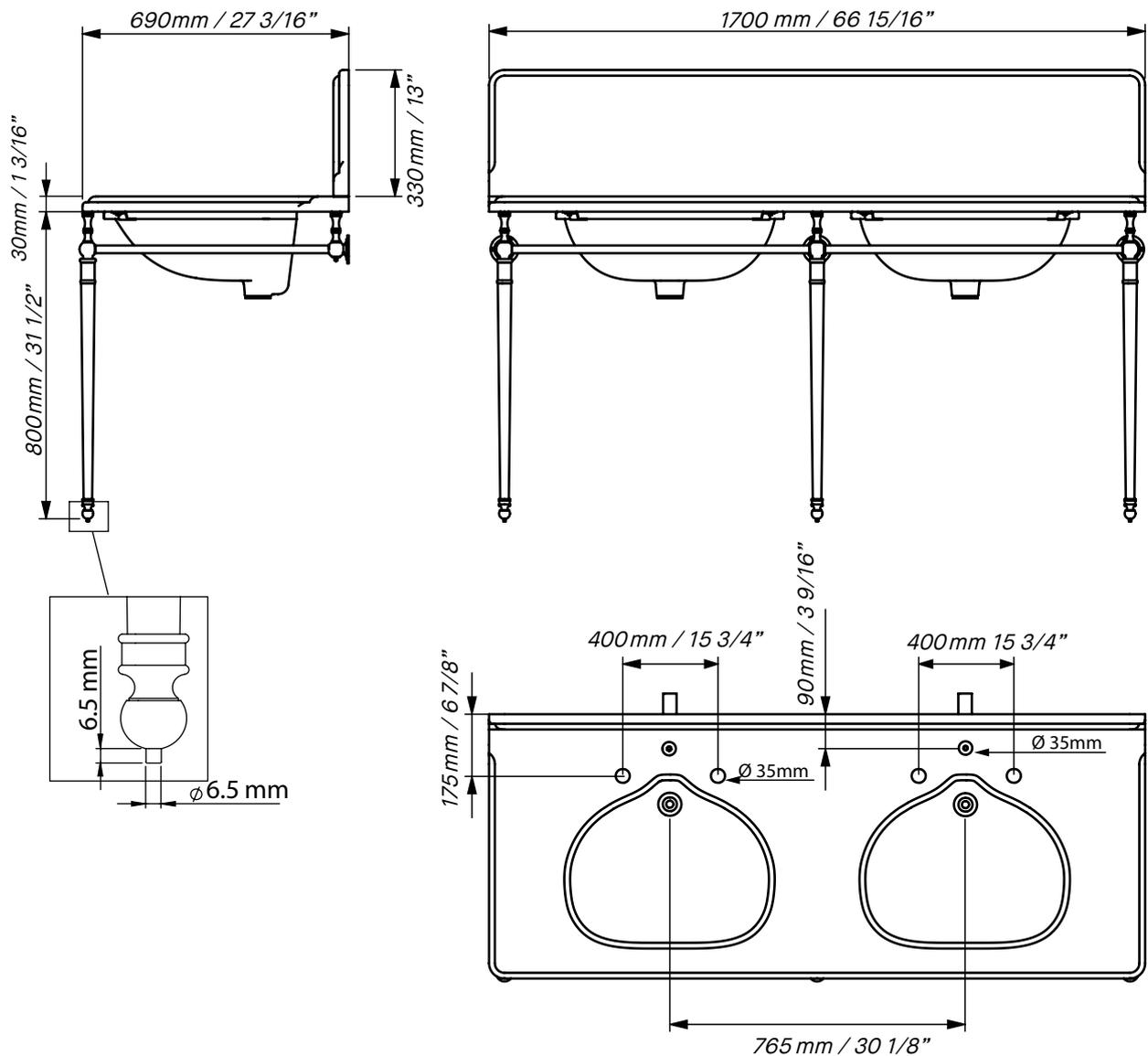
Height from floor to centre of waste outlet in wall should be between 450-480mm. Please note this is a guide height, using a Drummonds Waste and Bottle Trap
