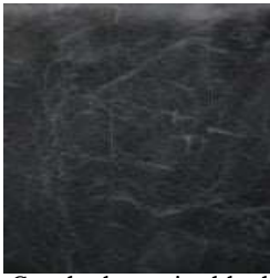
Cracked wax jet black
