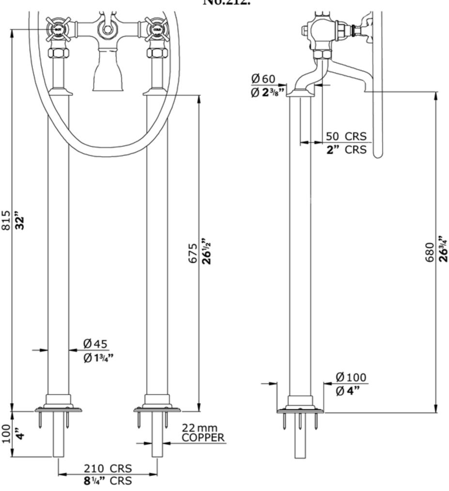
Cranked unions between standpipes and mixer body can be brought together or moved apart, so standpipe centres can be reduced to 5"/125mm minimum or expanded to 11"/280mm maximum.
